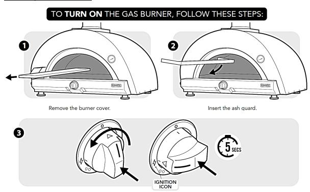
Press the knob and turn it to the ignition icon. Keep the knob pressed for 5 seconds.
