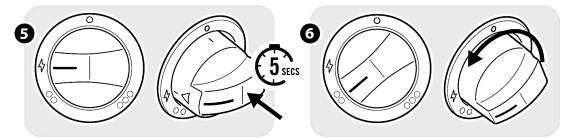
After lighting the pilot flame, hold the knob down for an additional 5 seconds to activate the thermocouple.
