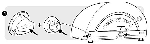
While keeping the knob pressed, press the igniter button at the same time to light the pilot flame.
