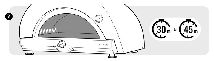
Allow the oven to preheat the bricks for 30 to 45 minutes before using the oven for pizza.
