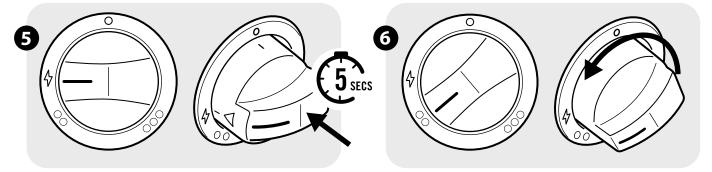
After lighting the pilot flame, hold the knob down for an additional 5 seconds to activate the thermocouple. Release the knob and turn it counterclockwise to activate the burner.
