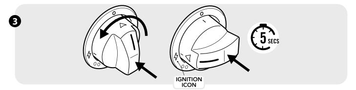
Press the knob and turn it to the ignition icon. Keep the knob pressed for 5 seconds.
