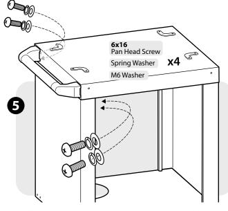
Finally, Attach the handle to the cart using the screws and washers provided. (4 – 6x16 Pan Head Screw, Spring Washer, M6 Washer)
