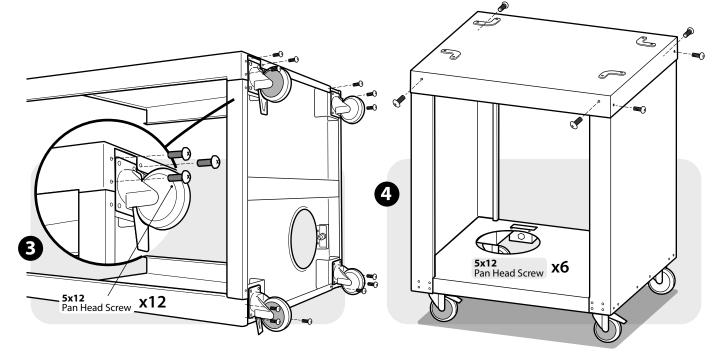
Install screws under the cart as shown. If needed, lay the cart on the side to complete this step. (12 - 5x12 Pan Head Screw)
