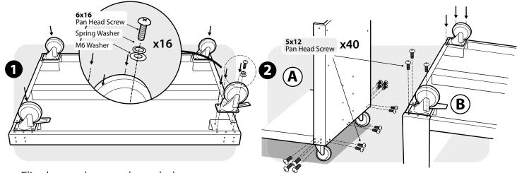
Flip the cart base and attach the casters with the locking casters at the front using the provided screws and washers.
