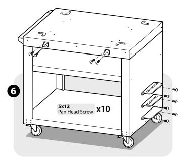
Finally, attach the tool holder and brackets to complete the assembly.
