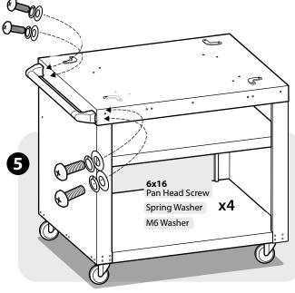
Attach the handle to the cart using the screws and washers provided.
