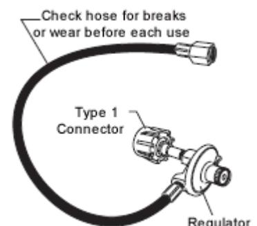
the flow of gas to 10 cubic feet per hour.
